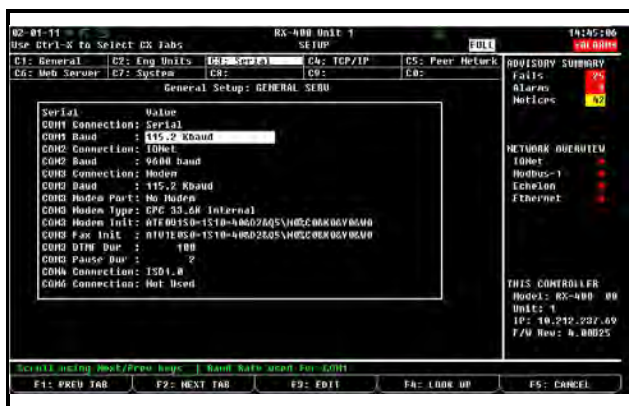
Figure 10-19 - I/O Network Baud Rate Setup
