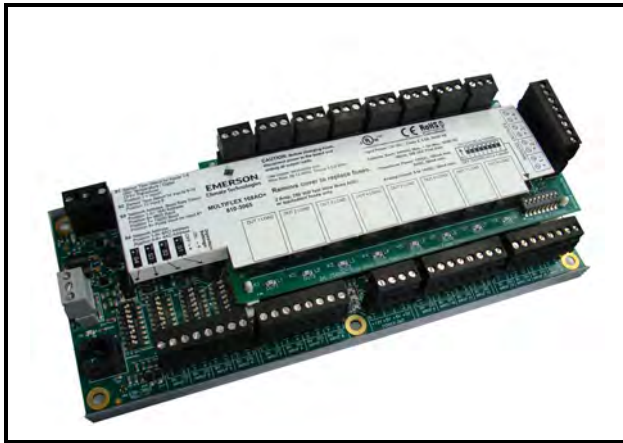
Figure 2-7 - MultiFlex Combination Input/Output Board (Side View)
