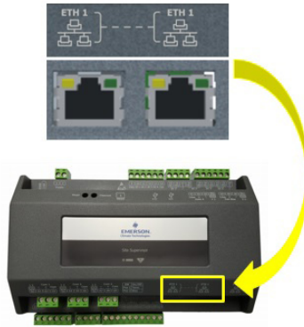
Site Supervisor ETH 1 Ports
