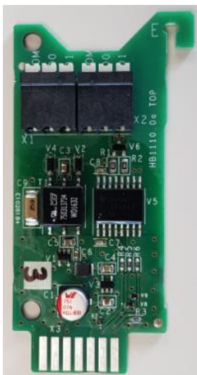
Figure 2: Modbus extension module E
