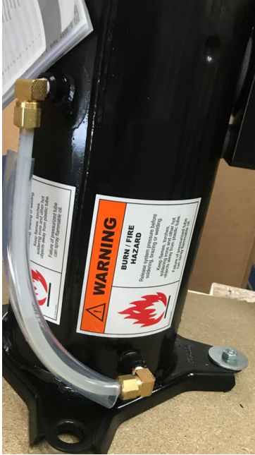
Figure 19: Sample compressor with external oil sight tube
