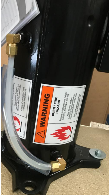
Figure 21: Sample compressor with external oil sight tube
