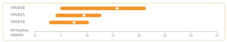
Conditions: Heating kW evaporating -7°C, condensing 50°C, 4K subcooling, 5K superheat
