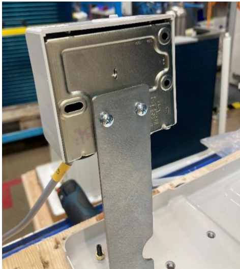
Figure 6: PS1 connected to the bracket
