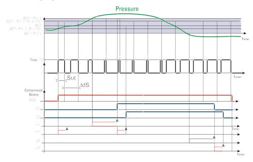
The capacity of the DGS compressor is limited by the PM and PMA parameters.
