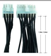
The EC2-XC645CX is provided with 2 socket connectors with 14 and 6 pins.
