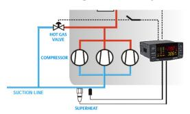
To detect the suction superheat an auxiliary probe among P3 (term. 3 - 4) or P4 (term. 27 - 28) has to be set as superheat temperature probe.
