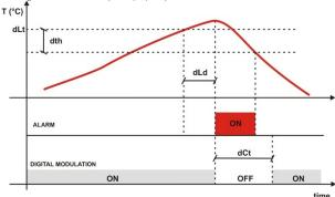
Until alarm delay time (dLd) is active the total compressor capacity will be limited to Cdd.
