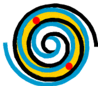
Figure 2: Position of the injection ports in the scroll set and the internal tubing connecting the injection inlet with the scroll set
