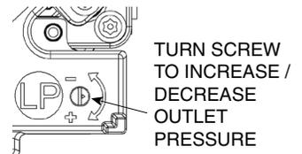
Fig. 5 – 36H27 Pressure Fine Adjustment
