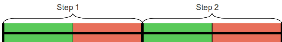
Figure 6-9. VFD Two-Step Control Method
