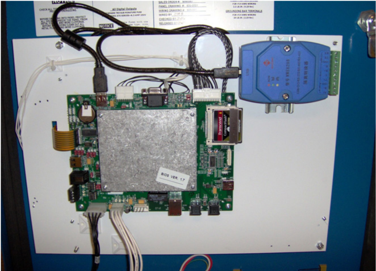
Figure C-2. Vision 20/20 Single Board Computer with USB to RS422/RS485 Converter (VPN3485C) on USB port P18
