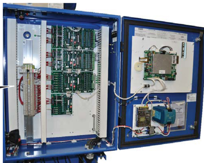
Figure 4-6. Wire Connections for Capacity and Volume Actuators
