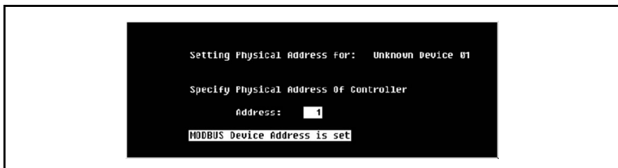
Figure 4-6 - Modbus Device Address is Set
