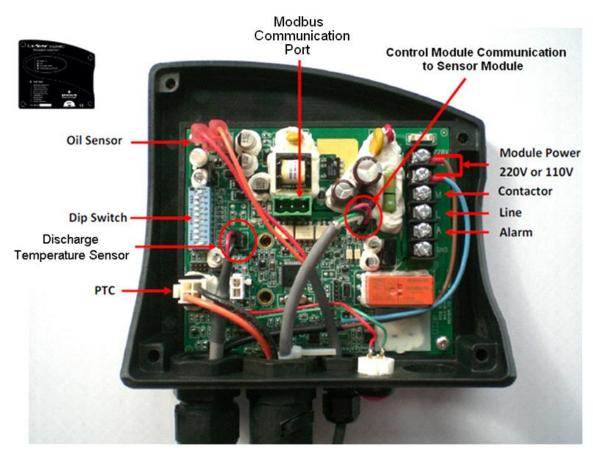
Figure 8: CoreSense wiring terminals description
