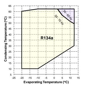
Figure 3: Inverter operation with standard motor 30 to 70 Hz - R134a
