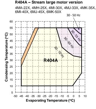
4MU-25X 60 55 50 Condensing Temperature (°C)  $\mathcal{S}$ 45 -60 HI 40 35 30 R404A 25 20 15 10 5 0 -50 -45 -40 -35 -30 -25 -20 -15 -10 -5 -55 0 Evaporating Temperature (°C) 0°C Suction Gas Return 20K Suction Superheat 25°C Suction Gas Return
