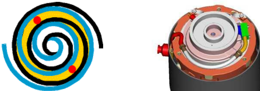
Figure 7: Position of the injection ports in the Scroll set and position of the internal tubing connecting the injection inlet with the Scroll set
